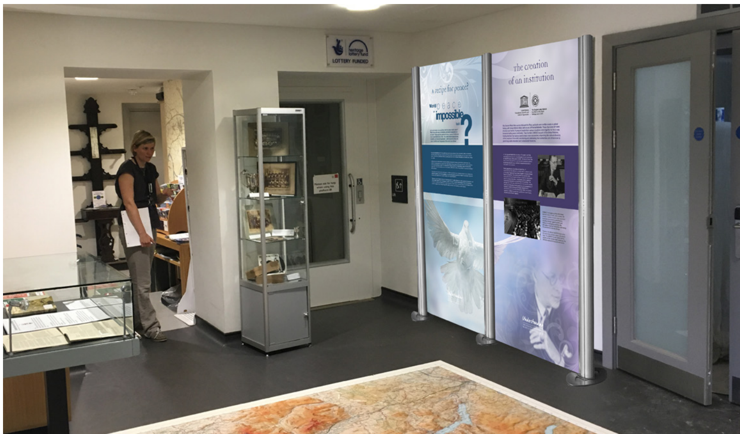
Example of aluminium furniture - Designed for temporary exhibitions, easily built and broke down. Being modular it can be built in several configurations. This example shows the display standing in front of the radiator on the wall.
